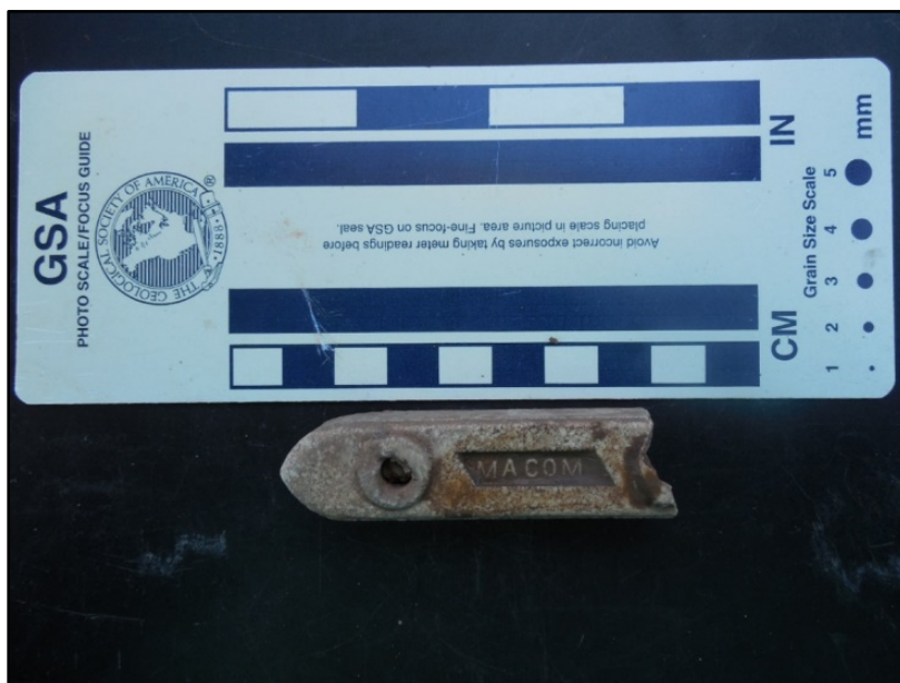
Figure 4.20: Macomb Cleat Insulator
