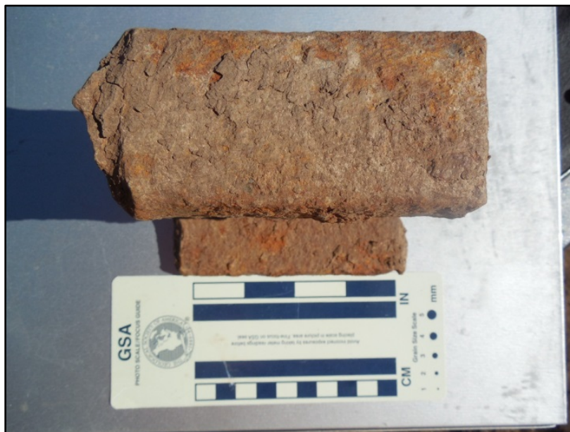
Figure 4.18: Portable Tram Road Rail
