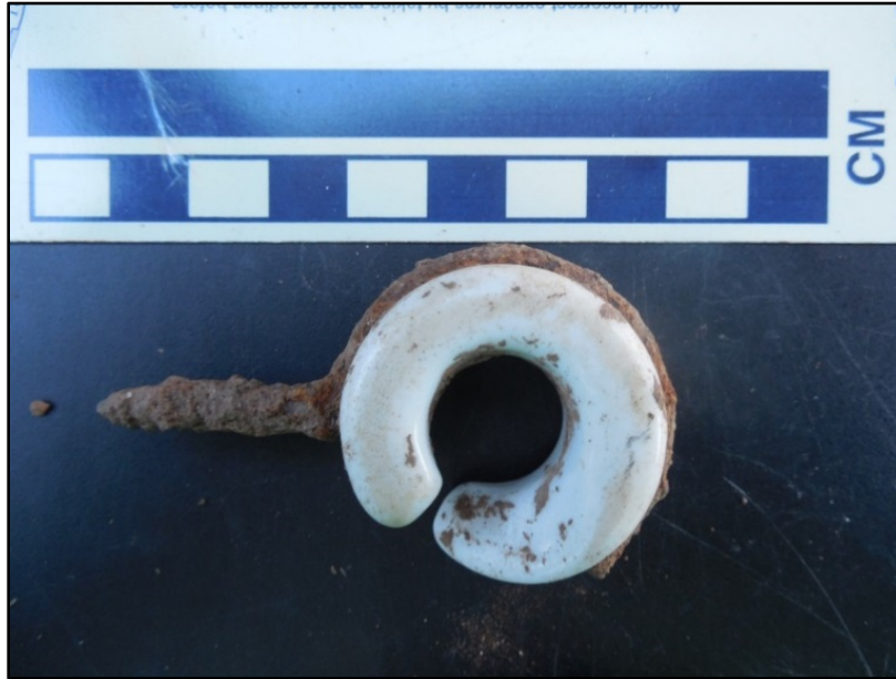
Figure 4.21: Bridle Ring Insulator for Telephone Drop
