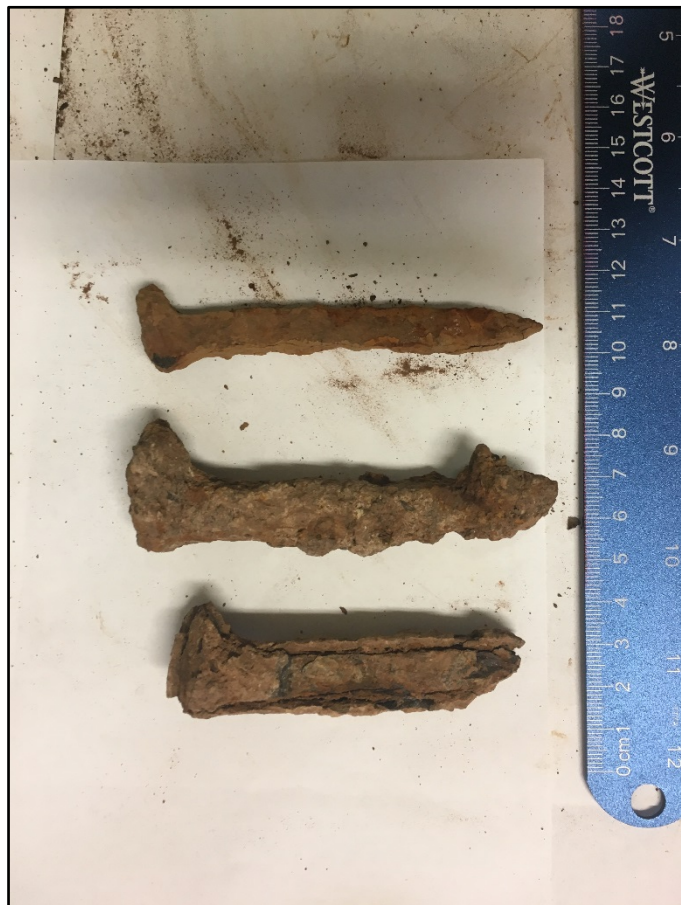
41FB355-22 Tie plate spikes, moveable sugarcane tram track
