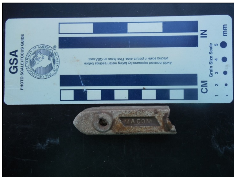
Figure 4.20: Macomb Cleat Insulator
