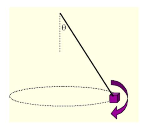
Object path is in the horizontal plane; Everywhere on the path, the net force is the same.
