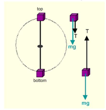
When the tension in the rope approaches zero...
