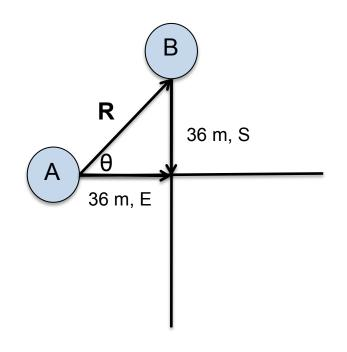
In this case, we need to find the position vector between car A and B. Since they happen to be the same distance from a reference point (the crossroad), it is sort of easy to see that the angle of B relative to A will be 45 deg (the x and y components of the position vector make a 45-45-90 triangle!)
