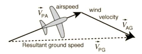
If the plane above is traveling with an airspeed of  $V_{PA}$  = 900 km/hr and encounters a wind speed of  $V_{AG}$  = 50 km/hr then what is the ground speed?
